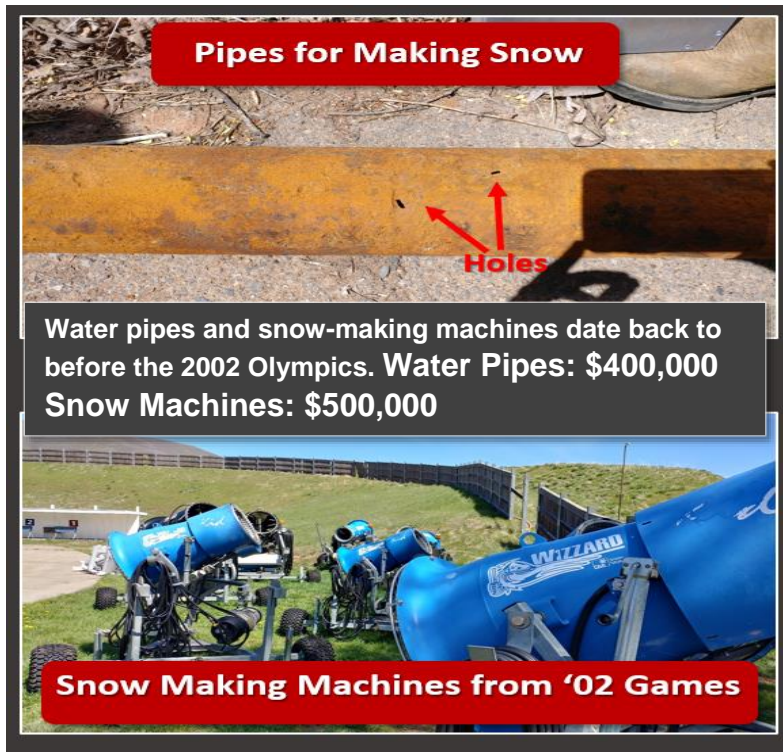
Figure 2.5 Soldier Hollow's Snow-Making Pipes Frequently Develop Holes. Part of the snow-making system is constantly shut off because of leaks.
