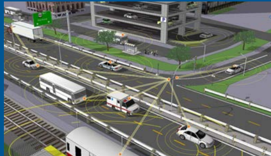
Connected vehicle communications
