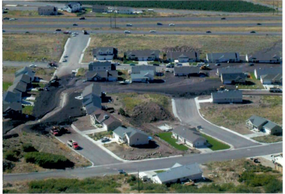
An intense rainfall-triggered debris flow that began in an area burned by a wildfire flowed through part of Santaquin in Utah County in 2002. The debris flow quickly inundated this Santaquin subdivision, leaving behind the dark, muddy deposits seen in this photo. (Photo credit: Dale Deiter, U.S. Forest Service)
