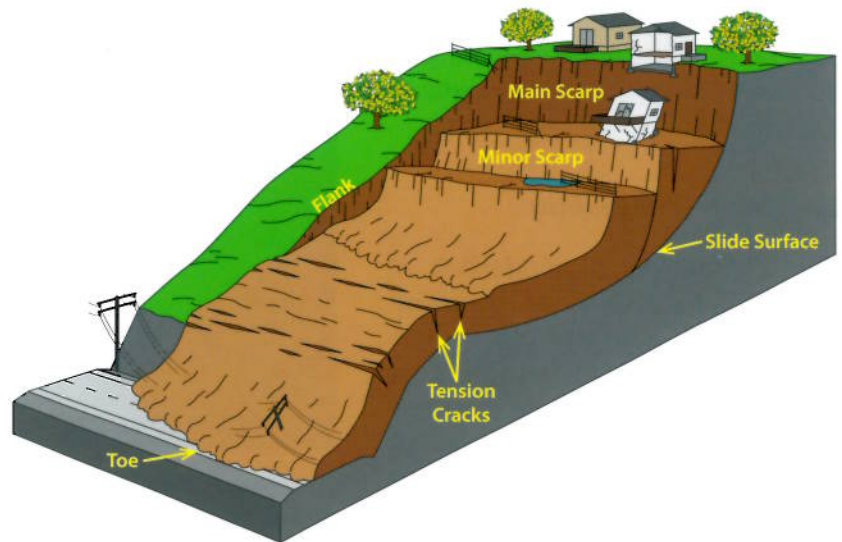
Diagram of an idealized landslide showing commonly used nomenclature for its parts.
