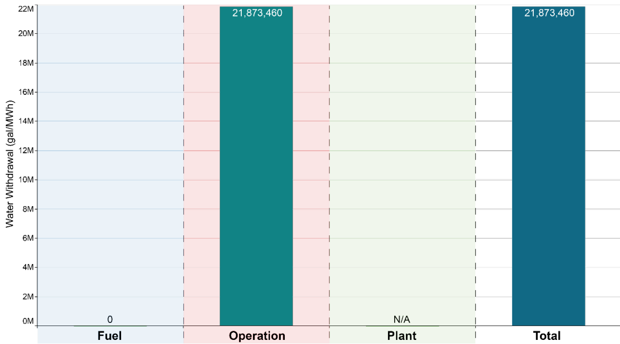
FIGURE 27: WATER WITHDRAWAL FOR ELECTRICITY GENERATION FROM HYDROPOWER
