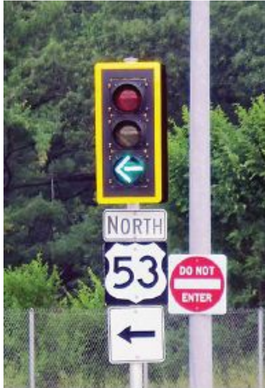
Example of a signal backplate framed with a retroreflective border.
