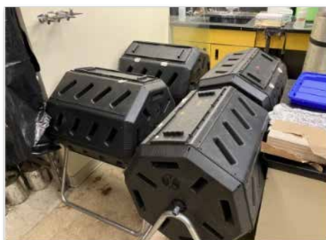
Figure 1: Laboratory composters used to evaluate the effectiveness of various treatments on PFAS transformation over time
