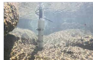
A pressure transducer installed in a rock glacier-fed stream in the Wasatch Mountains.
