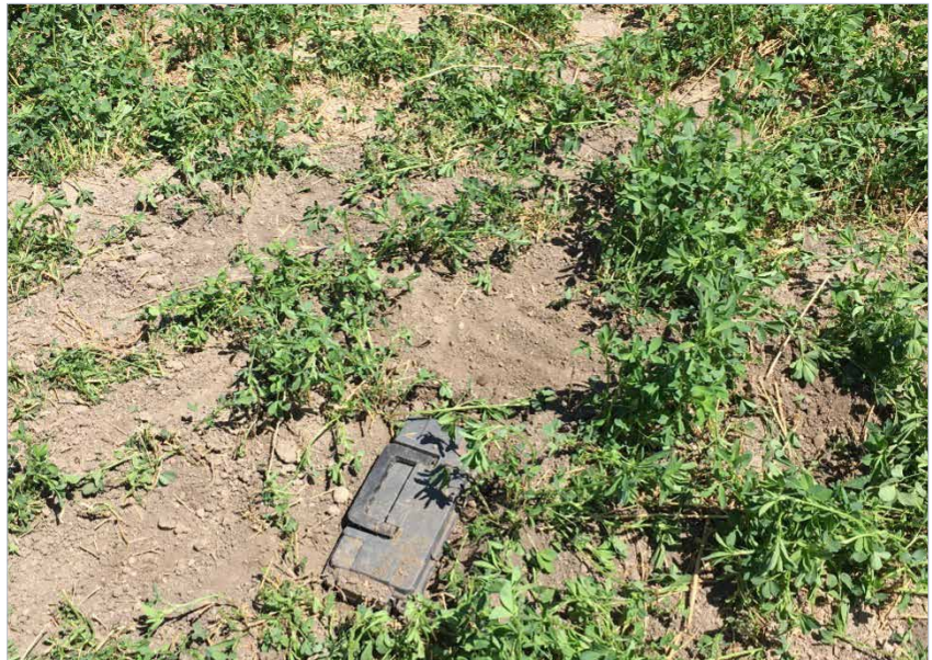
Figure 1: Soil moisture measurement site immediately after installation in one of the study fields
