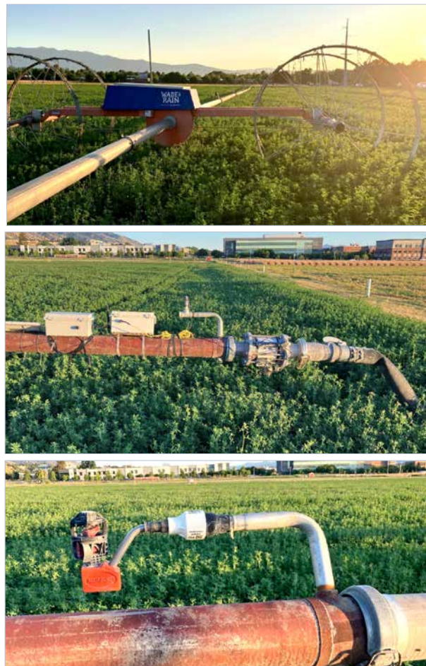
Figure 1: (top) Electric wheel line mover on a USU farm; (middle) Prototype automated shutoff and monitoring system on a wheel line at a USU farm; and (bottom) An example of a modern sprinkler technology being tested at a USU farm.
