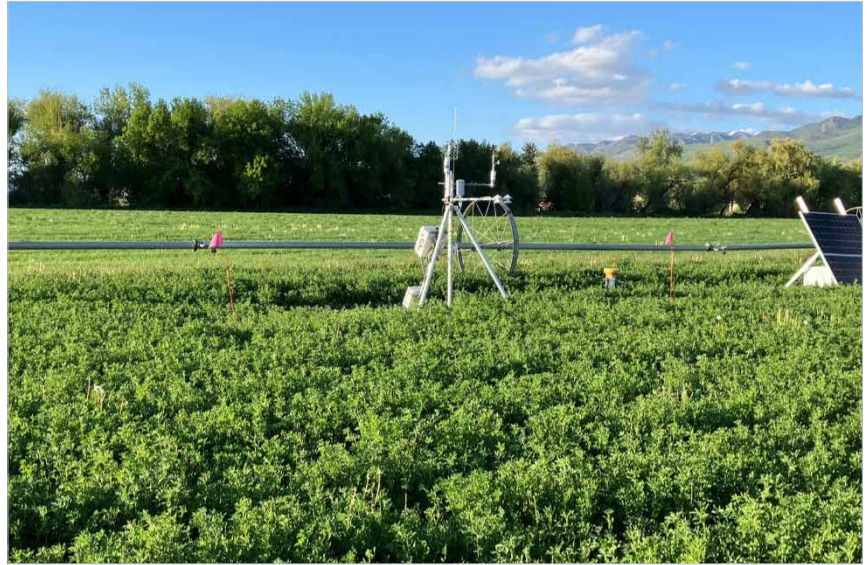
Figure 1: Eddy covariance measurement system installed at the edge of the SDI-irrigated alfalfa field (foreground) near Richmond, UT.
