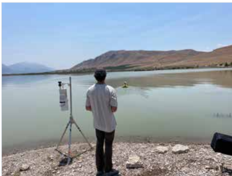
Figure 1: Air and water sampling to quantify the amount of cyanotoxins are in the aerosols generated off the surface of Utah Lake.
